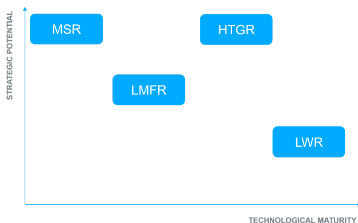
Figure 10: Positioning of SMR technologies over the axes strategic potential and technological maturity
