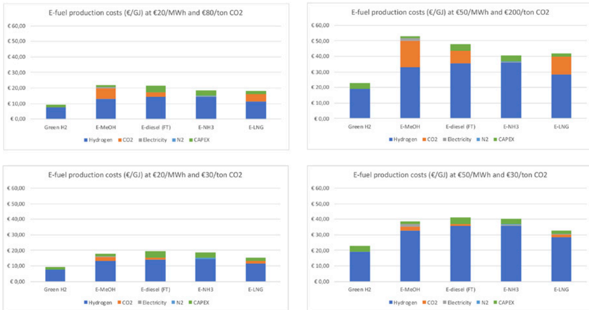
Figure 2 Production costs at different price levels for electricity and CO 2 . High CO 2 costs are associated with direct air capture and therefore dependent on electricity costs.
