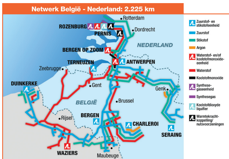
Figure 6. Hydrogen infrastructure of Air Liquide in North-Western Europe (AL, n.d.)
